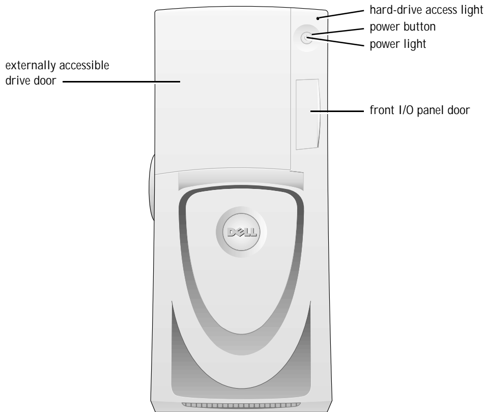
Front View of the Computer
